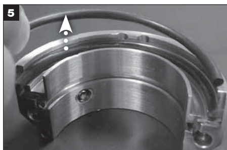
5 Remove used rotary face O-ring halves.
