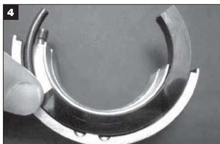
4 Remove used rotary face halves by pushing on end of face and sliding out of rotary holder half.
