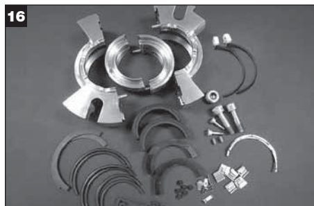
Remove all spare parts kit components from packaging and place on the clean work surface.
